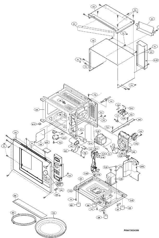
NOTE: In the event of removing the turntable motor cover this part should be refitted using screw connection: 50282957005 (7-10)
